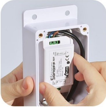
Place the switch into the housing and connect wires
