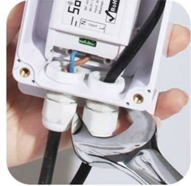
Fasten the wiring nuts with wrench until secure
